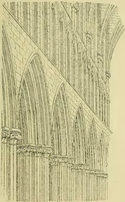
FIG. 120.—System of Nave of Wells.
